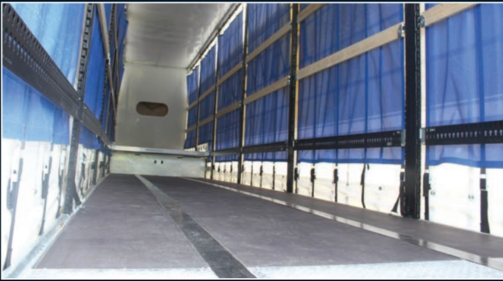
Sliding pillar and side cabbage boards
