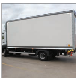
Fully bolted bodywork for ease of repair
