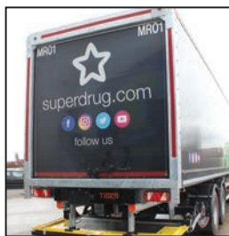
EN 12642-XL front, roof and rear frame assemblies
