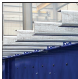
Galvanised floor bearers and aluminium alloy side rave with concealed fastenings
