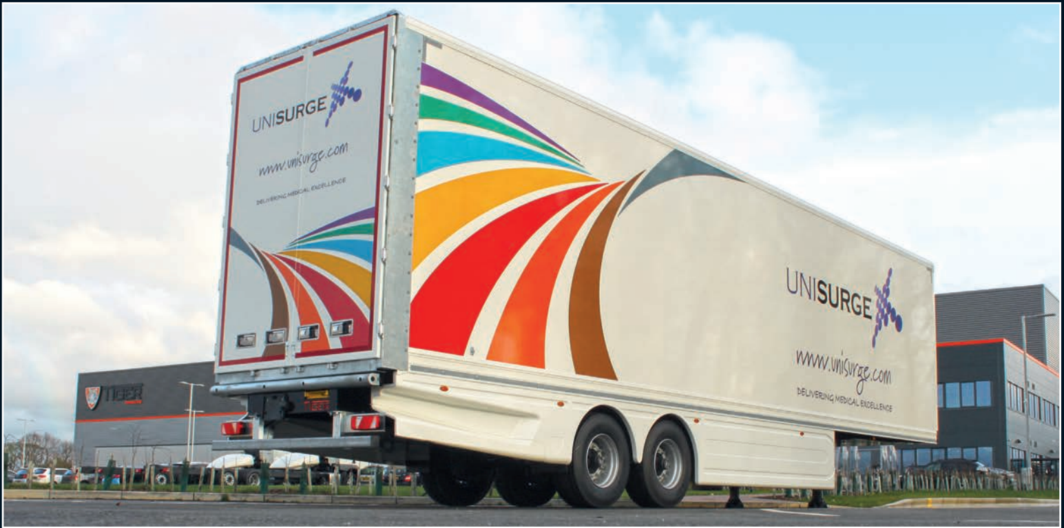
GRP aerodynamic sideguard system
