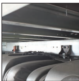
Galvanised chassis runners
