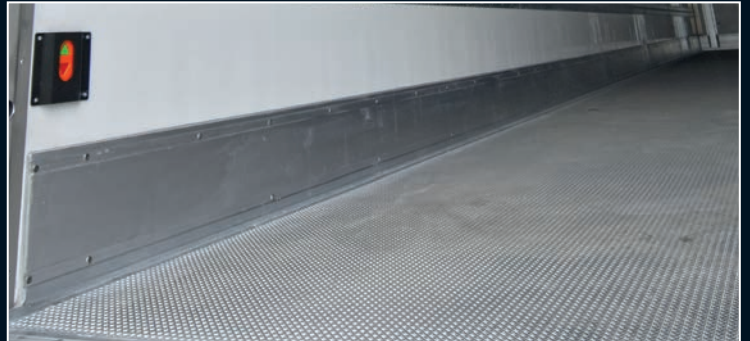
Aluminium floor for temperature-controlled trailers
