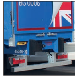
Hot-dip galvanised bolt-on under-run bar
