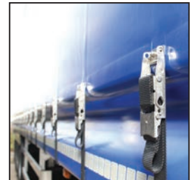
Stainless steel, bolt-on locking buckles
