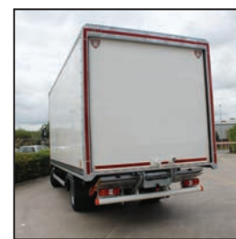
Hot-dipped galvanised rear frame with integral drain channel
