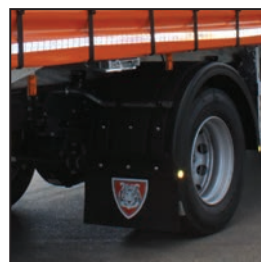
Thermo-plastic mudwings with spray suppression
