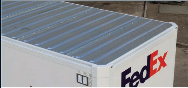
High security galvanised steel roof
