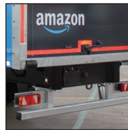
Hot-dipped galvanised under-run bar
