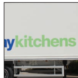
Pre-colour impregnated GRP side panels
